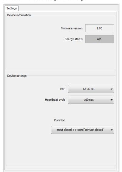
The device information shows the installed <u>Firmware version</u> and the current <u>Energy status</u> of the device.
